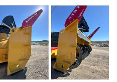
SIDE WING EXTENSIONS Allowing for cutting width extensions as well as overall stability and reinforcement to withstand abuse. Replaceable wear shoe.
